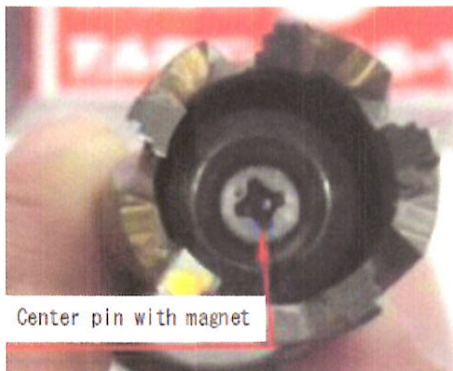
Figure 13. Drilling blade for trough rib
