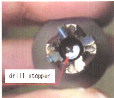
Figure 12. Drilling blade for deck side
